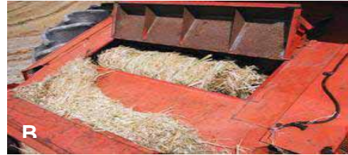
Hemp fibre clogging the cutting bar (A) and combine paddles (B, swathed).
